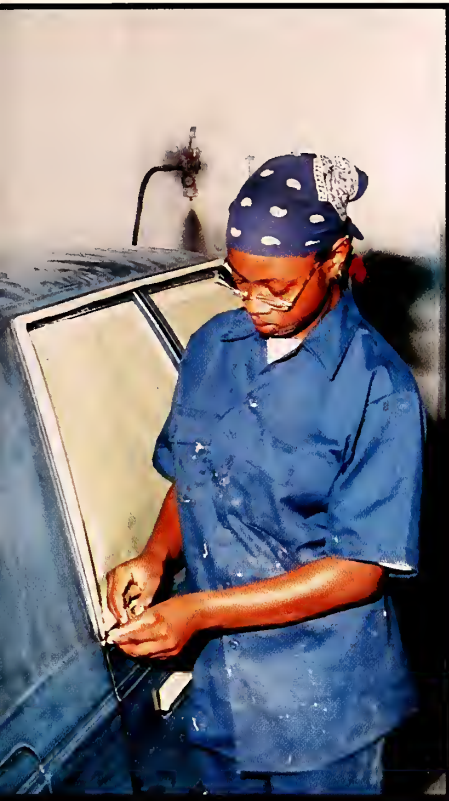
Cassandra is actually working. She is masking the areas of the car that are not to be painted.
