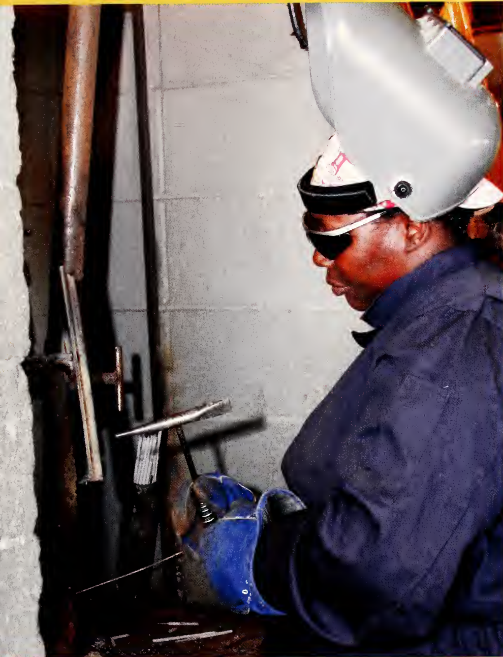
Left: Stacey Terrell does verticle fillet welding. She is from Utica and is the daughter of Utica Campus Police Chief Percy Terrell.
