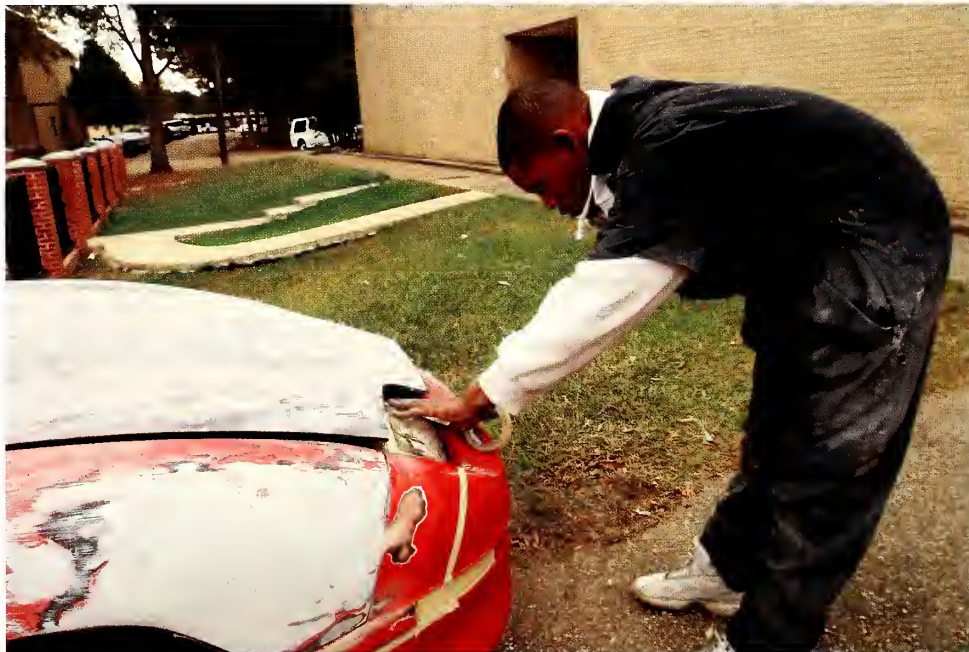
Kenderrian Beal tapes a Pontiac Sunfire before priming the car for paint. Beal is a freshman from Madison County.
