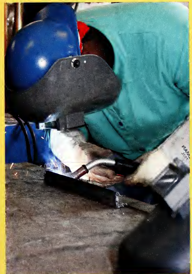
Above: Isiah McClure works to perfect the MIG welding, being careful to watch every bead.
