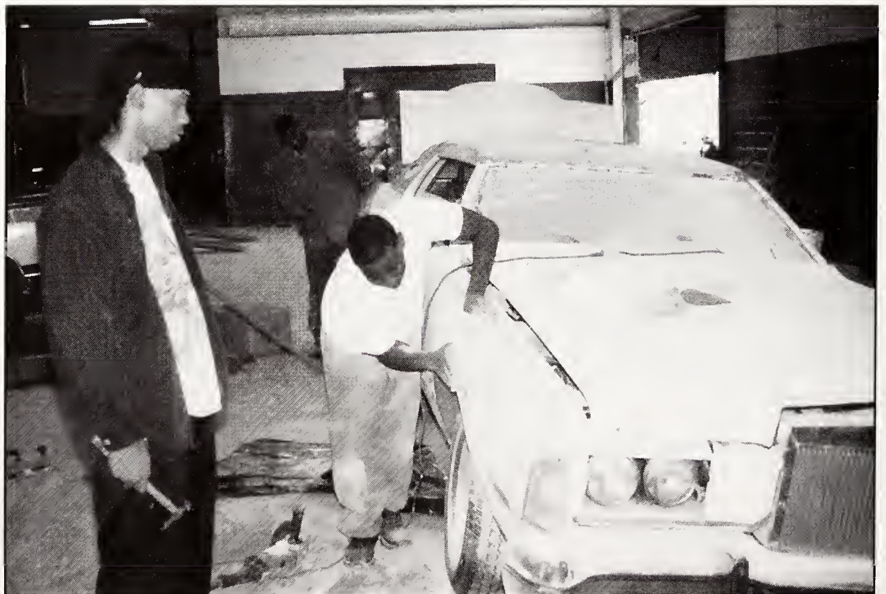
Leon Claiborne, Earl Christen, and Cory Kennebrew are shown sanding down rough areas on a 57 Lincoln Towne Car.
