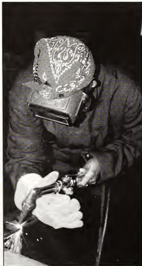
Gloria King is determined to master her skills at Oxyfuel Gas Cutting.
