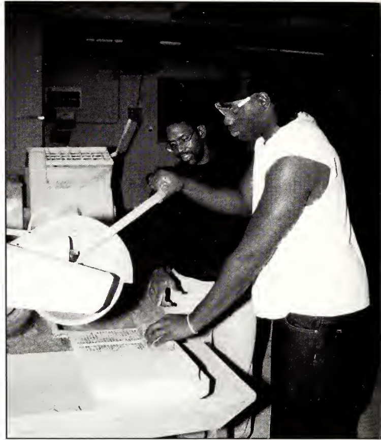
Instructor Mr. Rodney Warfield, back, shows student Derrick Hightower the proper way to cut bricks using a brick saw.
