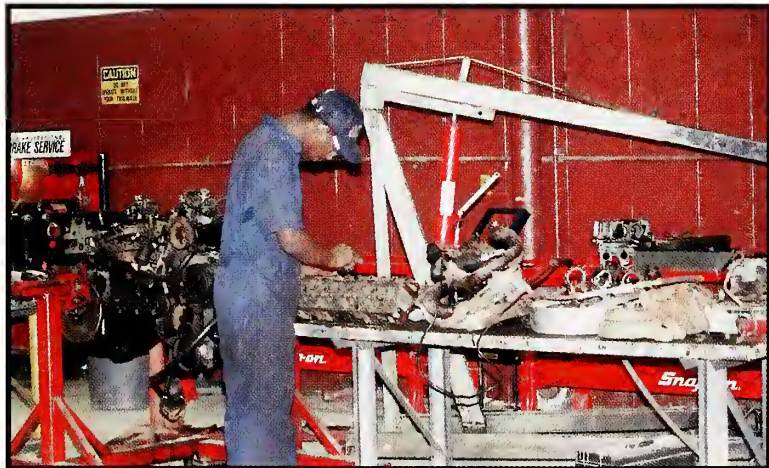
Dennis Mallory, a sophomore from Port Gibson, cleans the head of a 350 engine.
