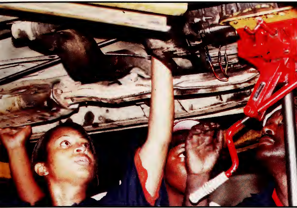
From left: Chealcey Wilson, Durell Hamilton, and Vernon Bozeman demonstrate their skills by installing a transmission into a Mazda truck
