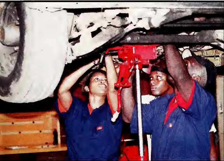
The team of Wilson, Hamilton, and Bozeman adds the finishing touch to securing the transmission.
