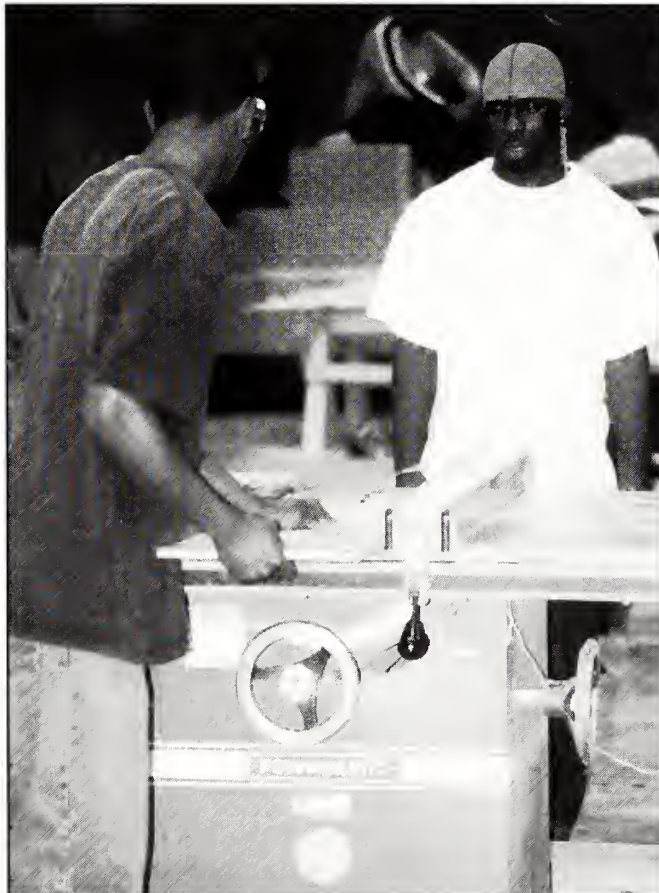
Tavarus Bates and Markea Byrd rip lumber to size using a table saw.
