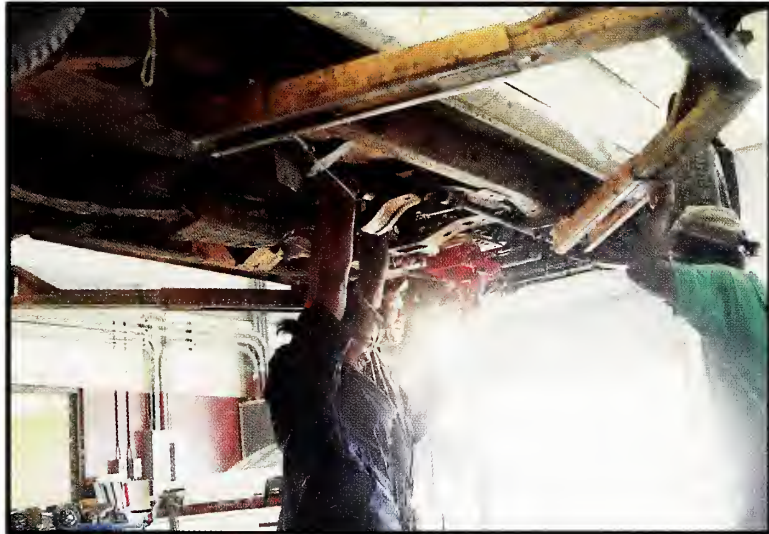
Chealcey Wilson and Vernon Bozeman work cooperatively to install a transmission as vehicle owner observes.
