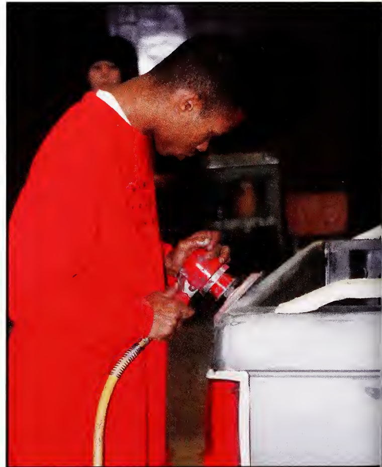
Vintorio Funchess, a sophomore from Crystal Springs, sands the truck before repairing the dents and rust spots.
