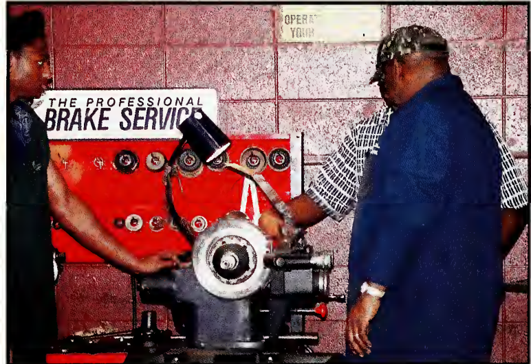
Cornelius Royal, left, and Deshon Rollins receive a first hand lesson from instructor, Mr. Stephen Murray, on how to turn rotors.
