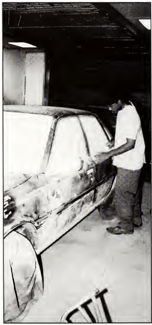
Auto Body students tape windows and other necessary parts of the car before painting.
