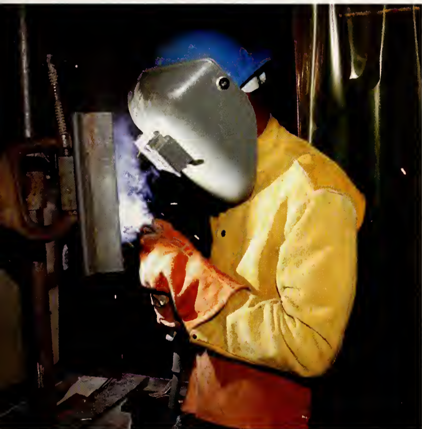
(above) LeShawn Warfield uses a flux cord to weld beads as a part of his practical learning. The instructor checks each bead for perfection.
