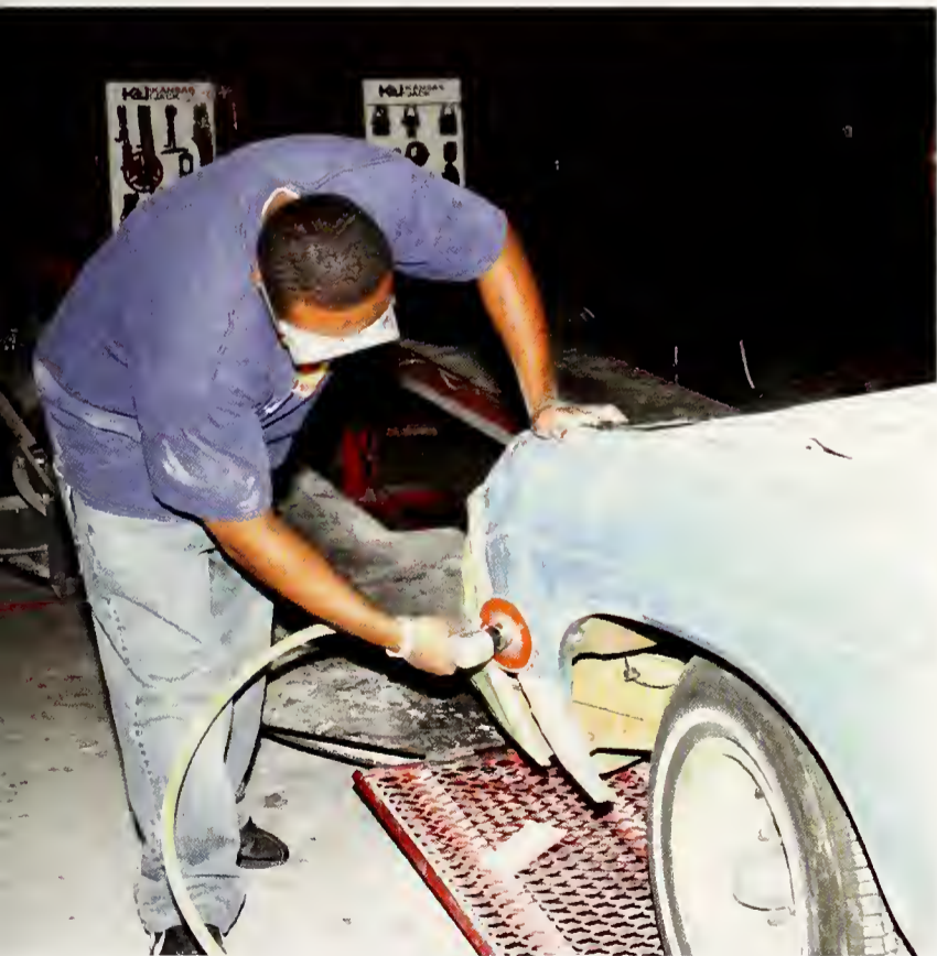
(above) Paul protects his eyes by wearing goggles as he grinds the front panel. Paul has taped the windows, bumpers, headlights and other parts of the car that will not require painting.
