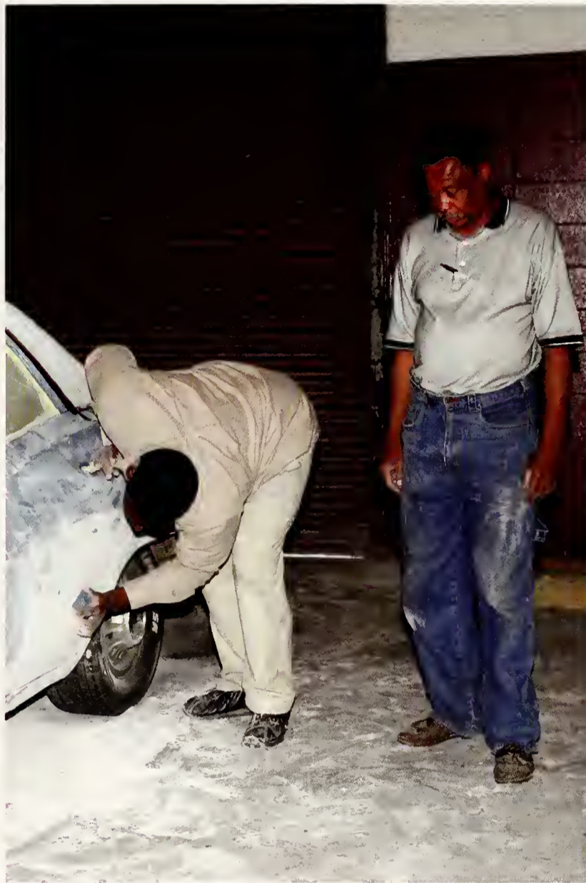
(below) Christopher Dampeer sands the side panel of the car before priming. Instructor Robert Jacobs observes and supervises.
