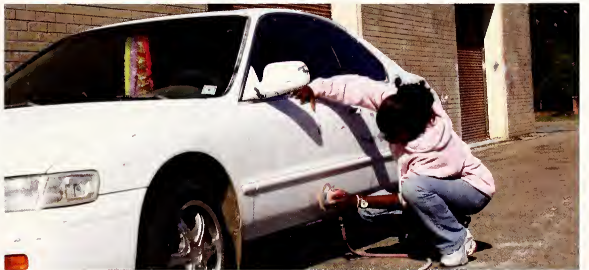
(above) LaTasha Miller sands the car as she prepares to paint. Prior to taking the car into the paint booth, the car has to be sanded, taped, primed, and have dents removed, if there are any.
