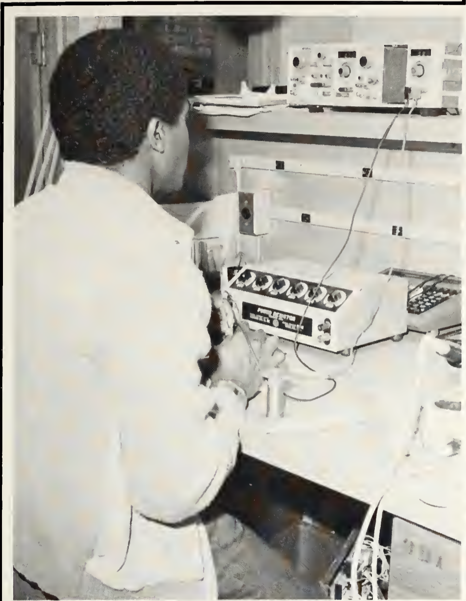
Ronald measures voltage in his trouble shooting efforts to repair the faulty device.
