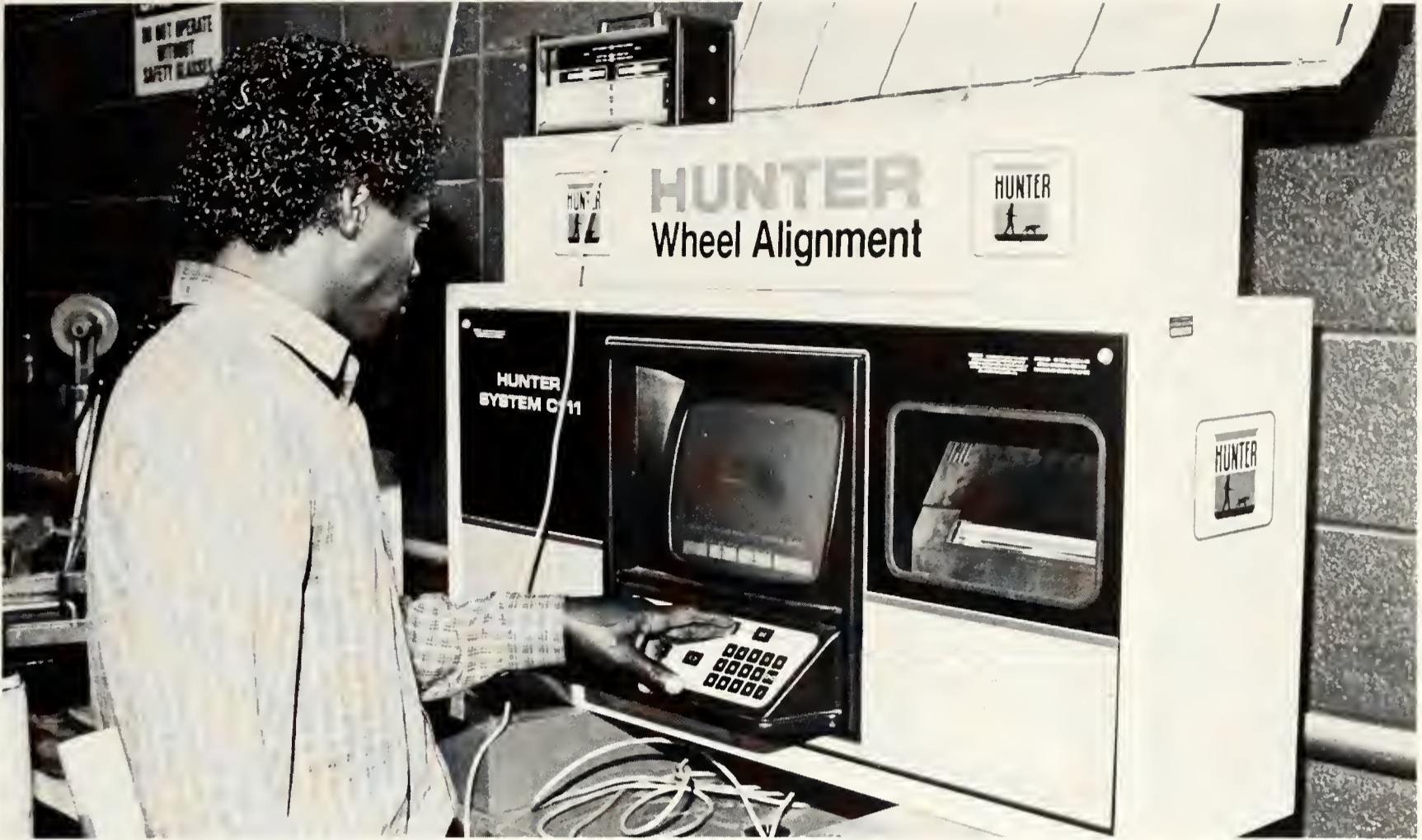
Andrew programs the computer to find out the exact alignment point of the wheel.
