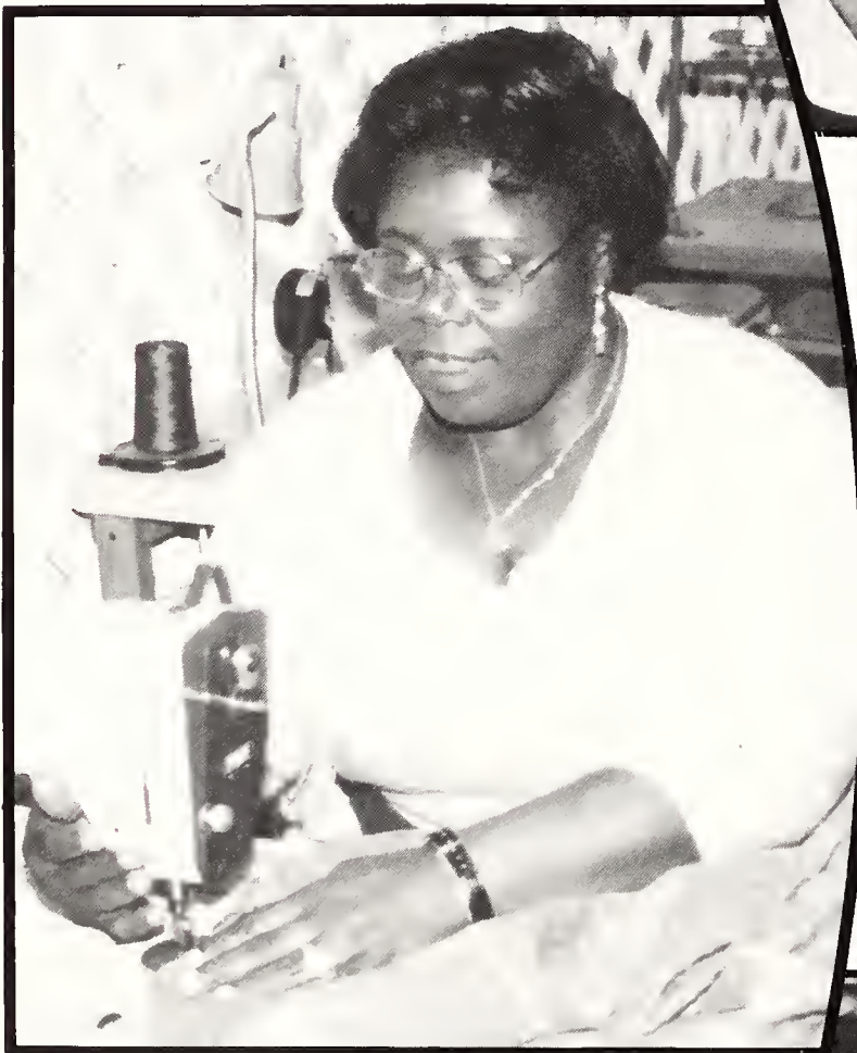
Mrs. Minnie Ether is using a blind stitch machine to hem an african garment.
