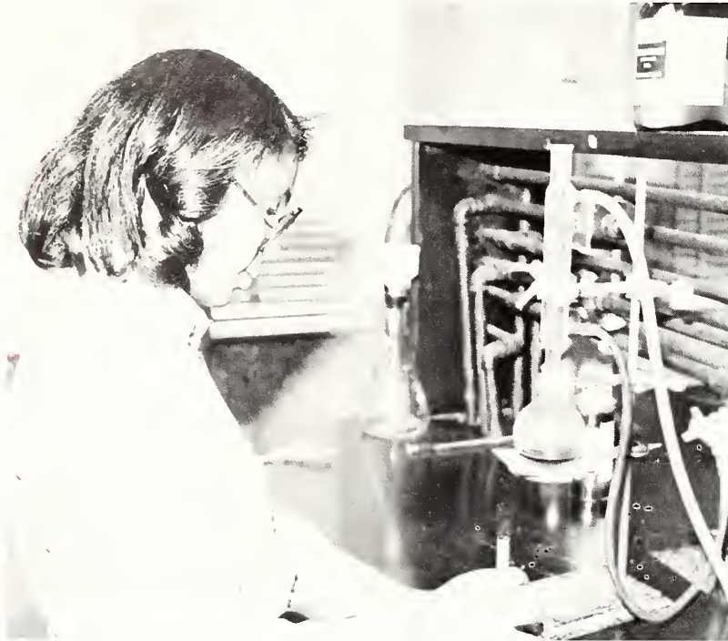
Cassandra works in the organic chemistry lab operating a reflux apparatus in the preparation of cyclohexane.
